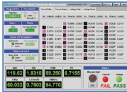
IEC 61000-3-2 Current Harmonics Test (Pre-compliance)
