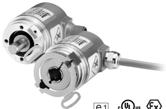
The Sendix M36 with Energy Harvesting Technology is an electronic multiturn encoder in miniature format, without gear and without battery. With a size of just 36 x 53 mm it offers a blind hollow shaft of up to 10 mm.
