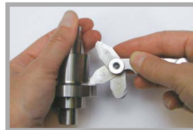
Measurement of radius using a convex radius gauge
