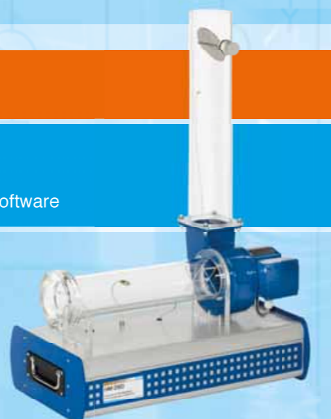
HM 280 Experiments with a Radial Fan
