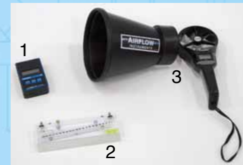
1 digital manometer, 2 inclined tube manometer, 3 anemometer
