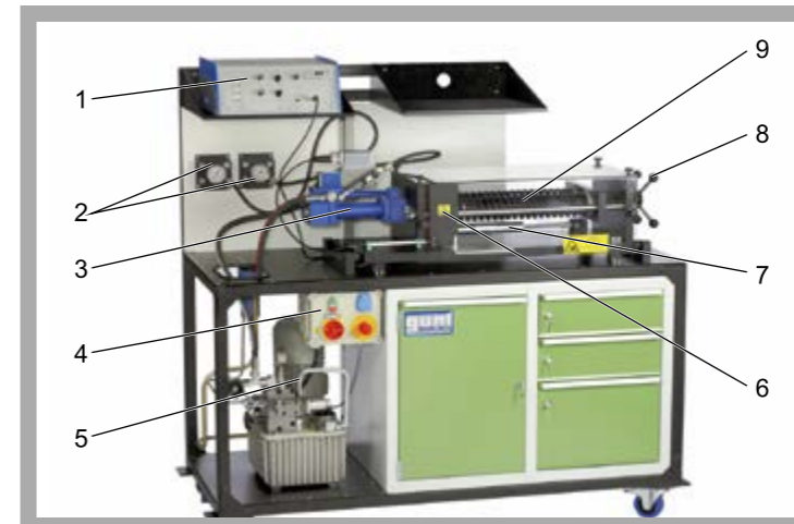
1 servo amplifier, 2 cylinder pressure manometer, 3 hydraulic cylinder with control valve, 4 switch box, 5 pump and oil tank, 6 carriage, 7 damper, 8 hand wheel for spring pre-tension, 9 springs
