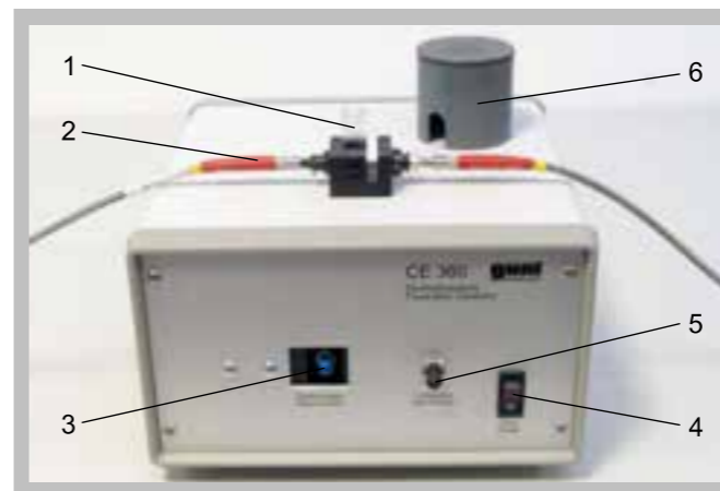
Photometer: 1 cell, 2 light conductor, 3 spectrometer connection, 4 main switch, 5 light source connection, 6 cap
