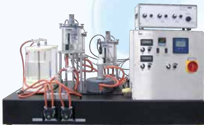
Supply Unit for Chemical Reactors CE 310 with Stirred Tanks in Series CE 310.03
