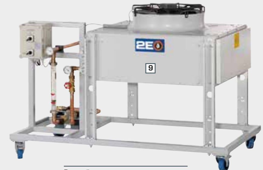
Dry cooling tower
