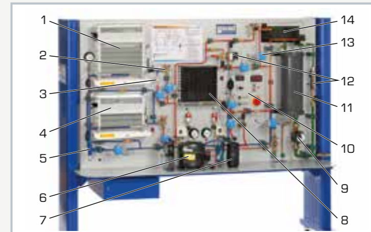
1 evaporator, 2 expansion valve, 3 capillary tube, 4 freezing stage evaporator, 5 evaporation pressure controller, 6 compressor, 7 receiver, 8 heat exchanger with fan, 9 pump, 10 display and control elements, 11 tank for glycol-water mixture, 12 flow meter, 13 solenoid valve, 14 coaxial coil heat exchanger
