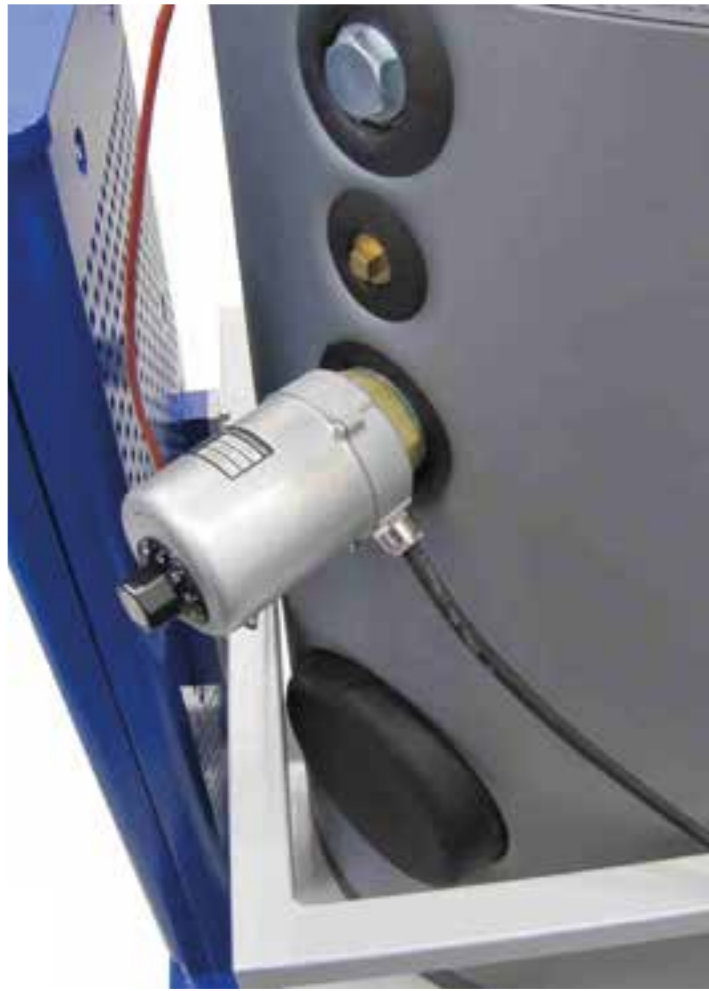
HL 320.02 heater installed in the bivalent storage tank of HL 320.05
