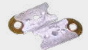
Trip element with melted solder joint
