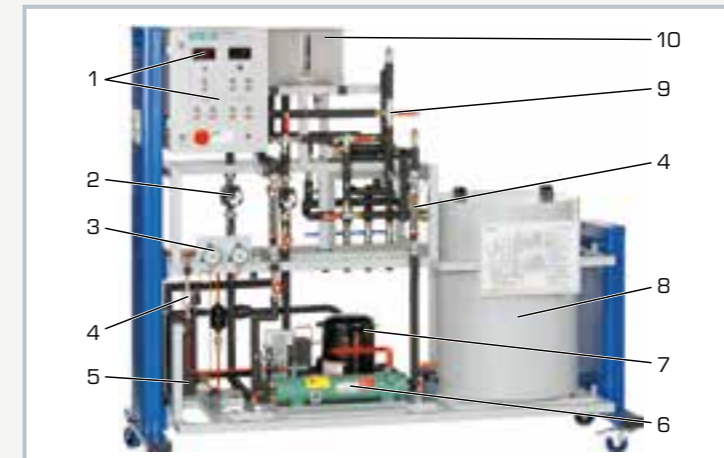
1 displays and controls, 2 pump, 3 manometer, 4 flow meter, 5 evaporator, 6 condenser, 7 compressor, 8 ice store, 9 3-way valve, 10 compensation tank (glycol-water mixture)
